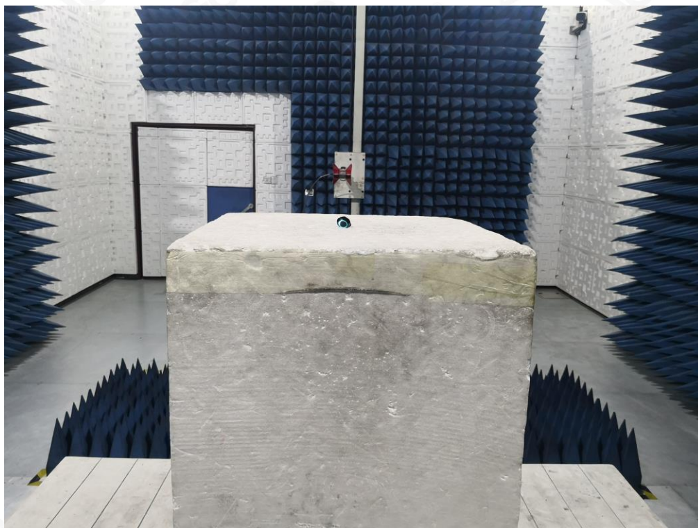
RADIATED EMISSION TEST SETUP ABOVE 1GHZ
