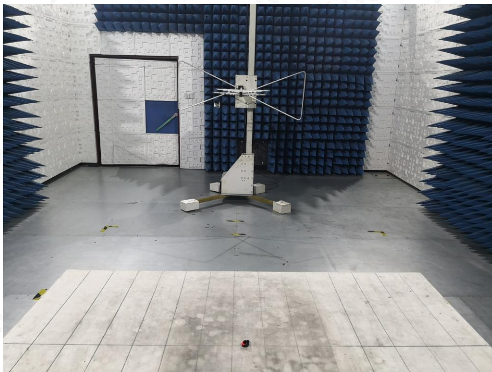
RADIATED EMISSION TEST SETUP ABOVE 1GHZ
