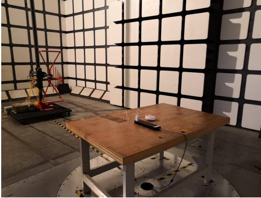
Radiated Emissions View (Below 1 GHz)
