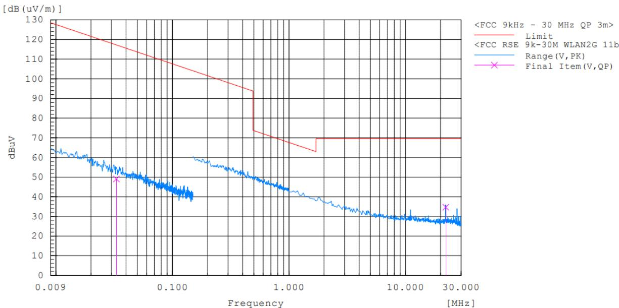
**Radiated Spurious Emission 9 kHz – 30 MHz (Antenna Position 180°)**
