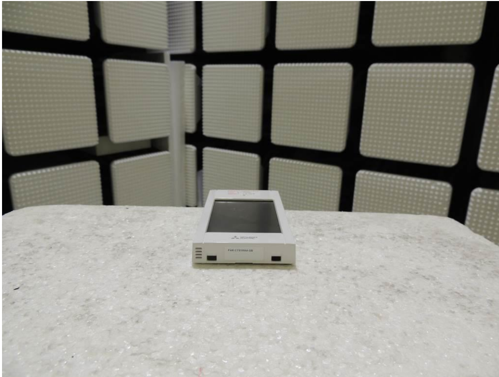
Photograph 6: Set-up for Radiated Emission, EUT Configuration X-Axis
