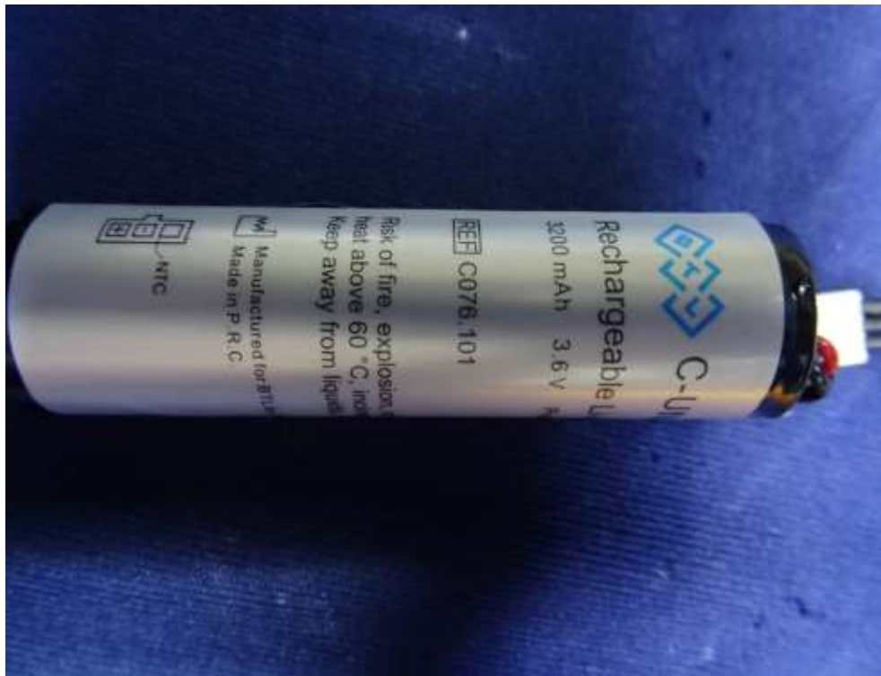
Internal battery ratings
