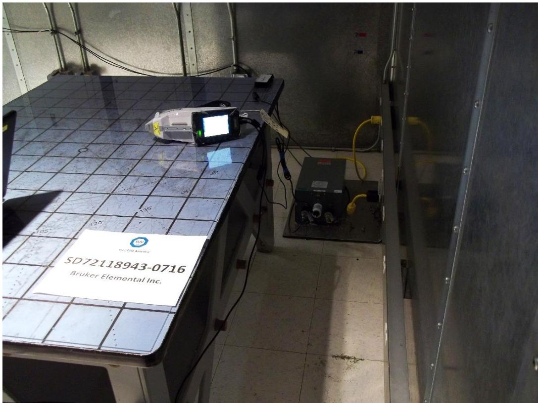
**Conducted Emissions Test Setup (Back)**
