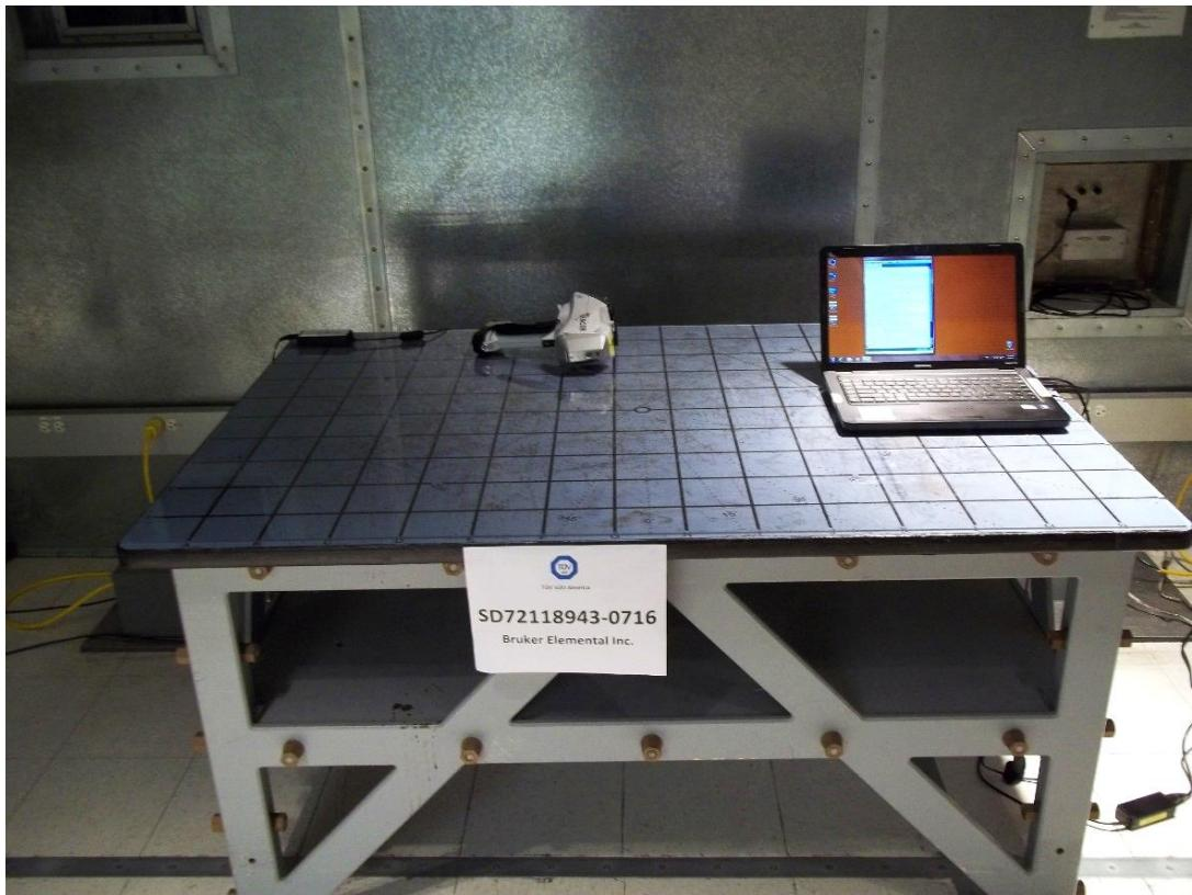
**Conducted Emissions Test Setup (Front)**
