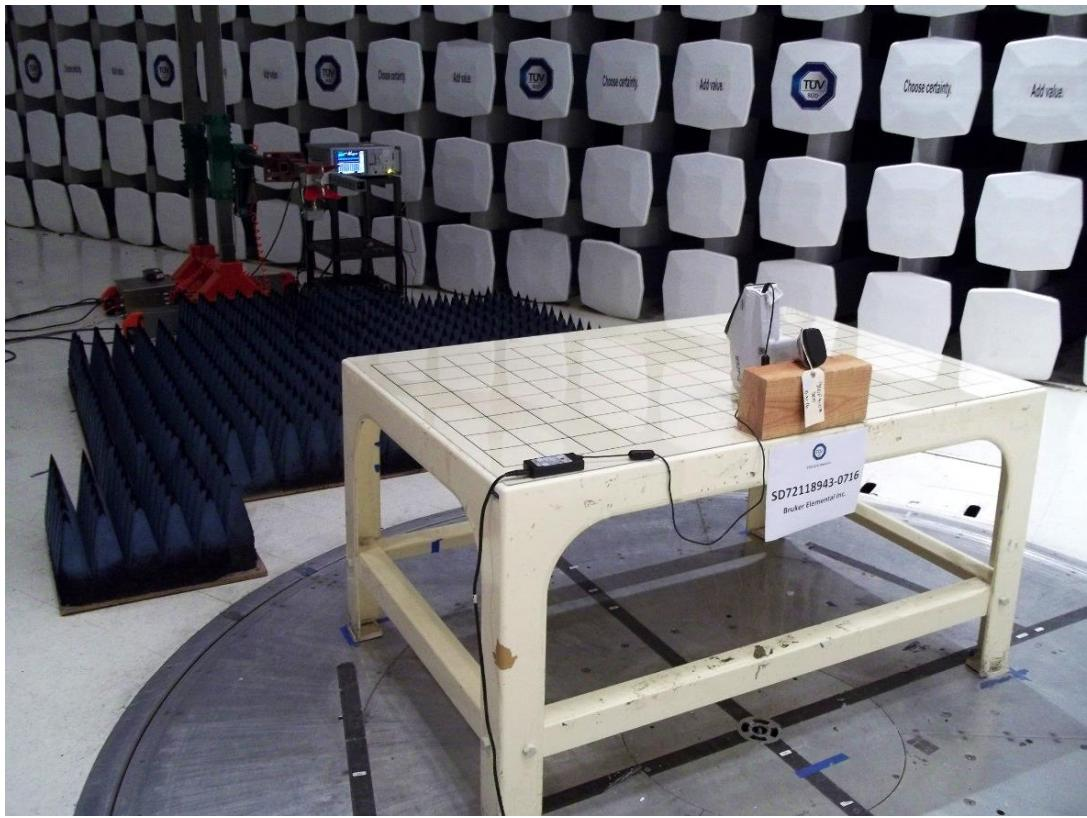
**Radiated Emissions Test Setup (above 1GHz Back)**
