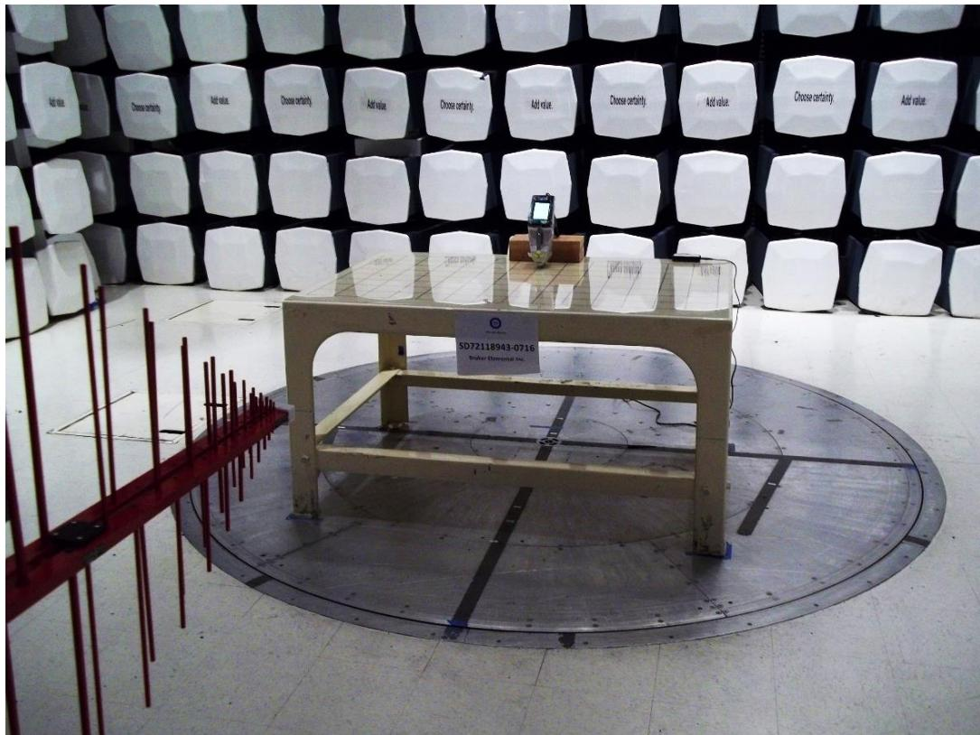
**Radiated Emissions Test Setup (below 1 GHz Front)**
