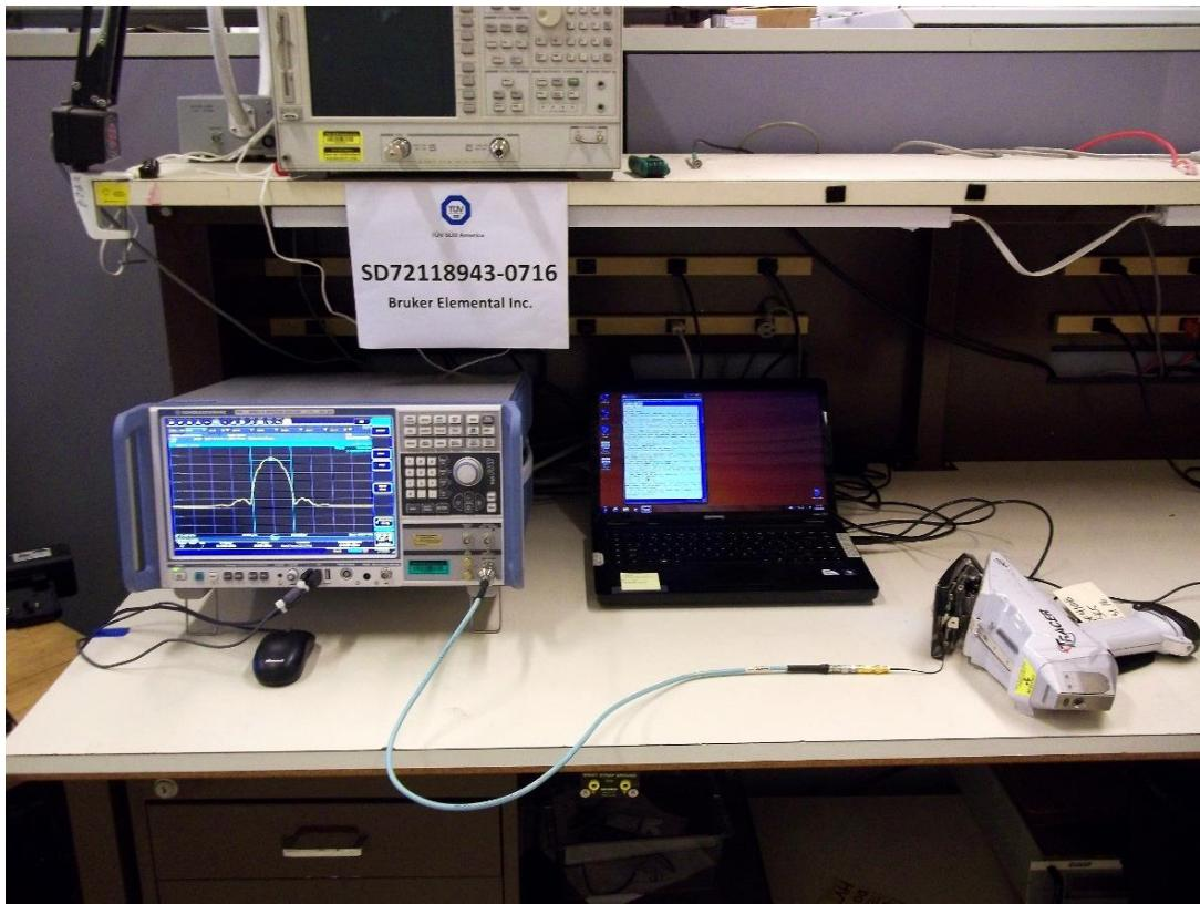
**Conducted Antenna Port Test Setup**
