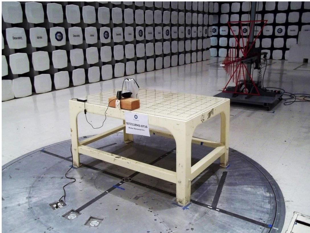
**Radiated Emissions Test Setup (below 1 GHz Back)**
