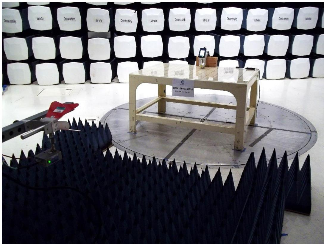
**Radiated Emissions Test Setup (above 1GHz Front)**
