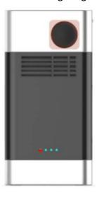
3. The indicator specification: the first lamp light, show that the product has power on, the second to the fourth lamp one by one flashing lighting shows in charging; All four lamp light up shows the battery is full, battery volume indicator is shown in figure.
