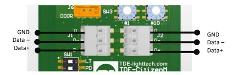
When connecting the Ethernet cable make sure that wires 3, 5 and 7 are connected together to reduce impedance. The same applies for wires 4, 6 and 8. In order to prevent voltage drop of the power supply voltage. Both connectors are parallel connected, in order to connect another module on the same bus.
