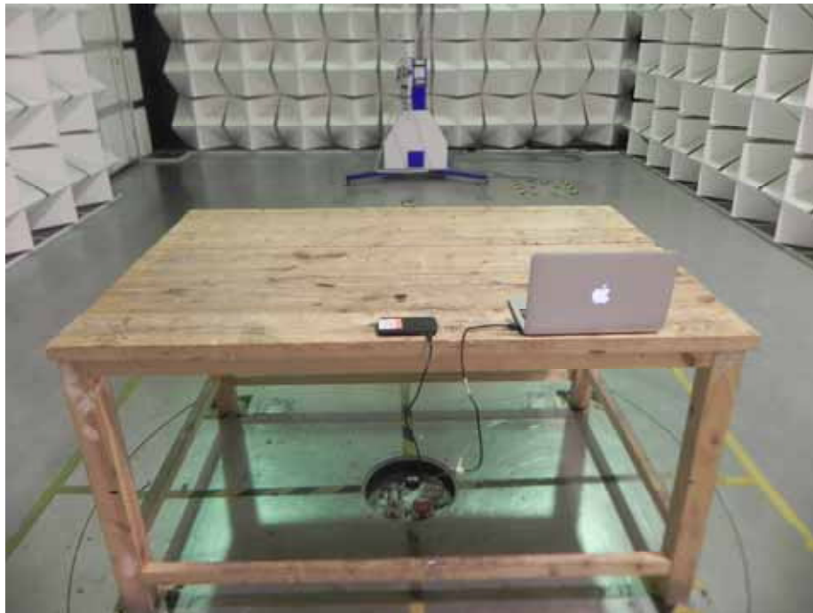
30MHz-1GHz at Test Site 2#
