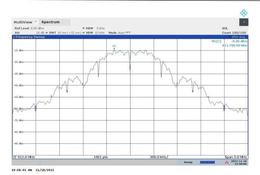
Graph7: 912MHz Lowest Channel 3 kHz PSD Plot
