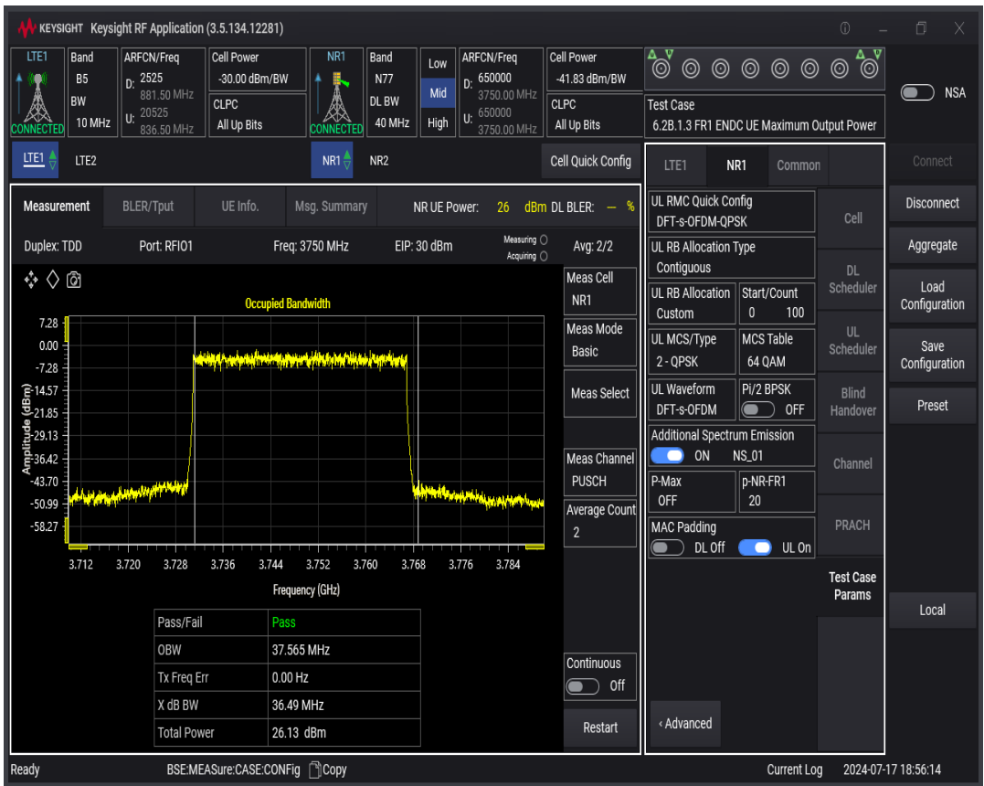
n77 SCS=30kHz DFT_QPSK BW=50MHz Channel=650000 RB=128@0
