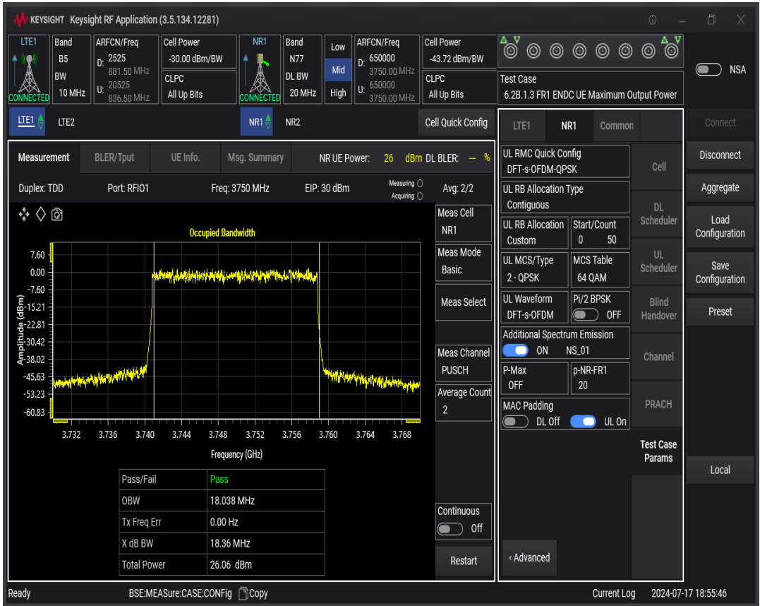
n77 SCS=30kHz DFT_QPSK BW=40MHz Channel=650000 RB=100@0
