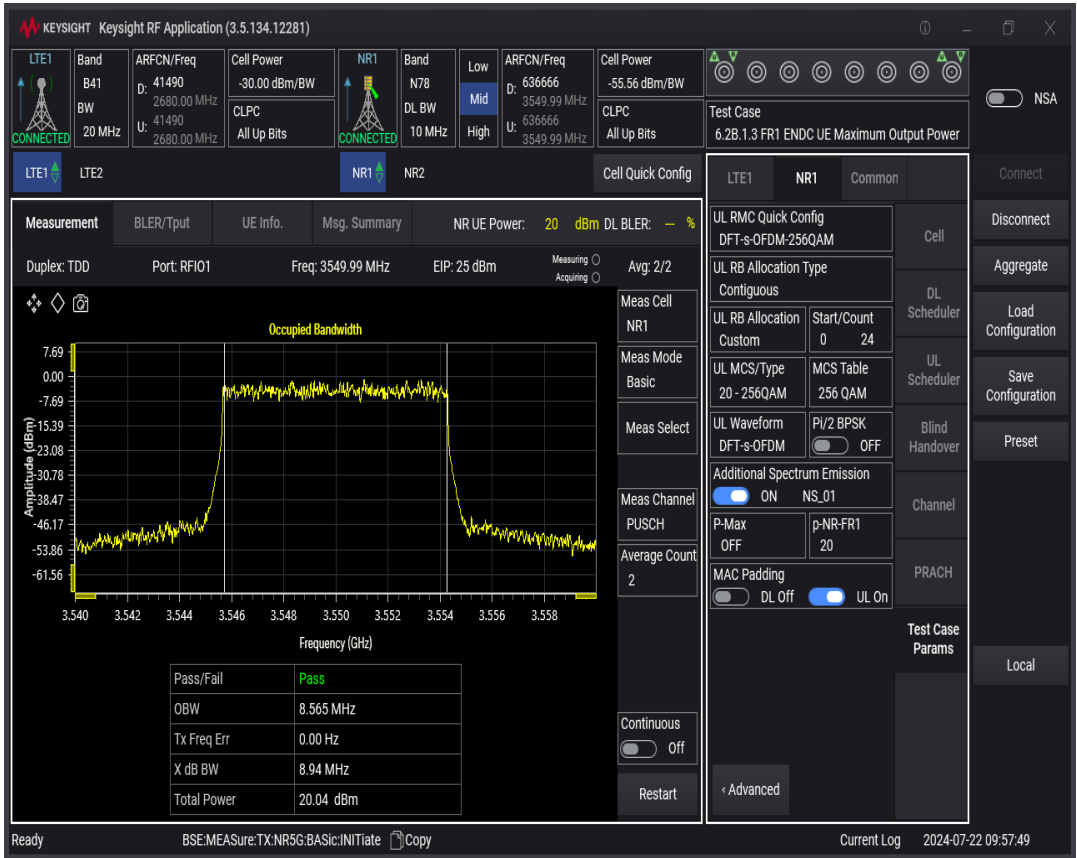
n78 SCS=30kHz DFT_QAM256 BW=15MHz Channel=636666 RB=36@0
