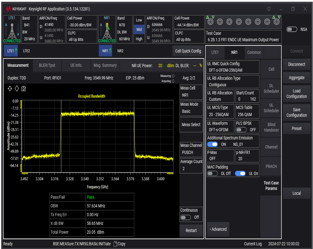
n78 SCS=30kHz DFT_QAM256 BW=80MHz Channel=636666 RB=216@0
