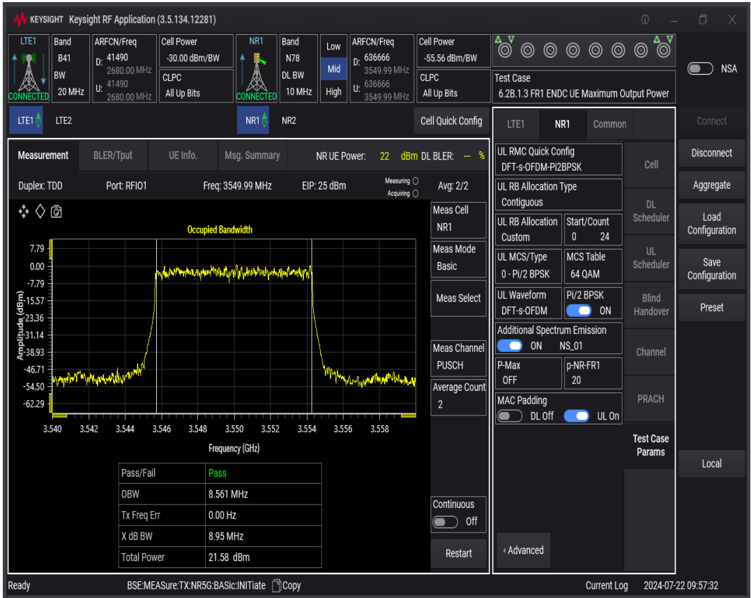
n78 SCS=30kHz DFT_BPSK BW=15MHz Channel=636666 RB=36@0
