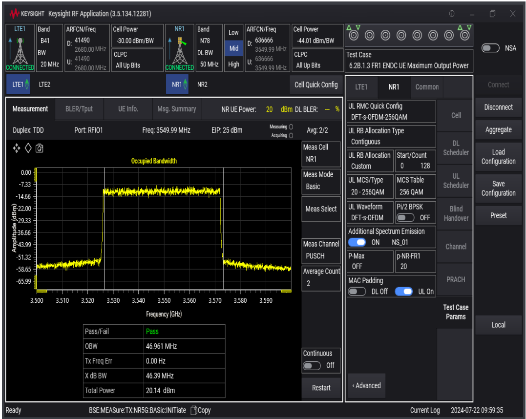
n78 SCS=30kHz DFT_QAM256 BW=60MHz Channel=636666 RB=162@0
