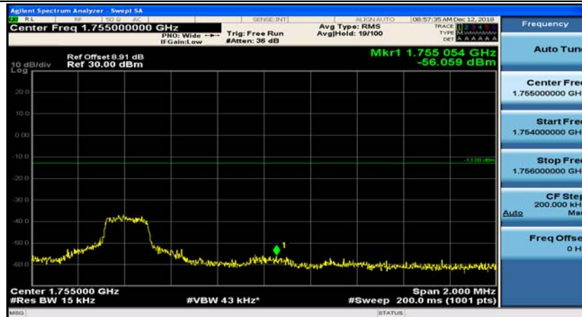
Channel Bandwidth: 10 MHz_HCH_16QAM_1RB#24
