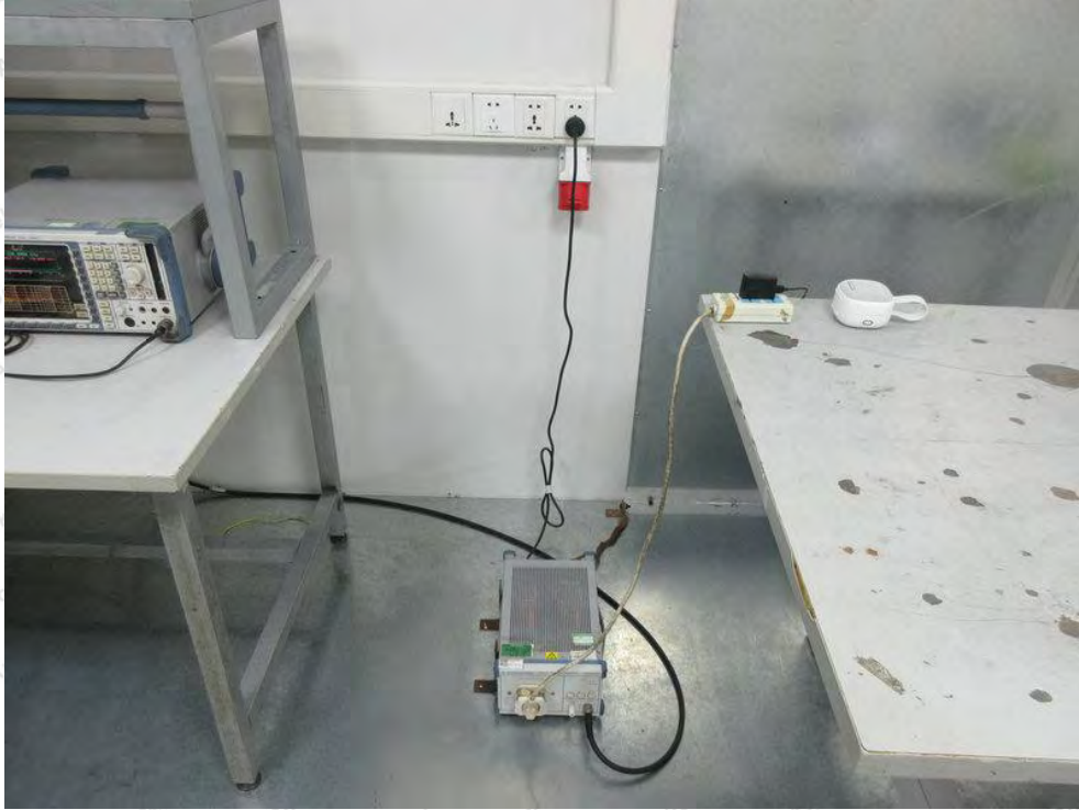
Photo of Conducted Emission Measurement
