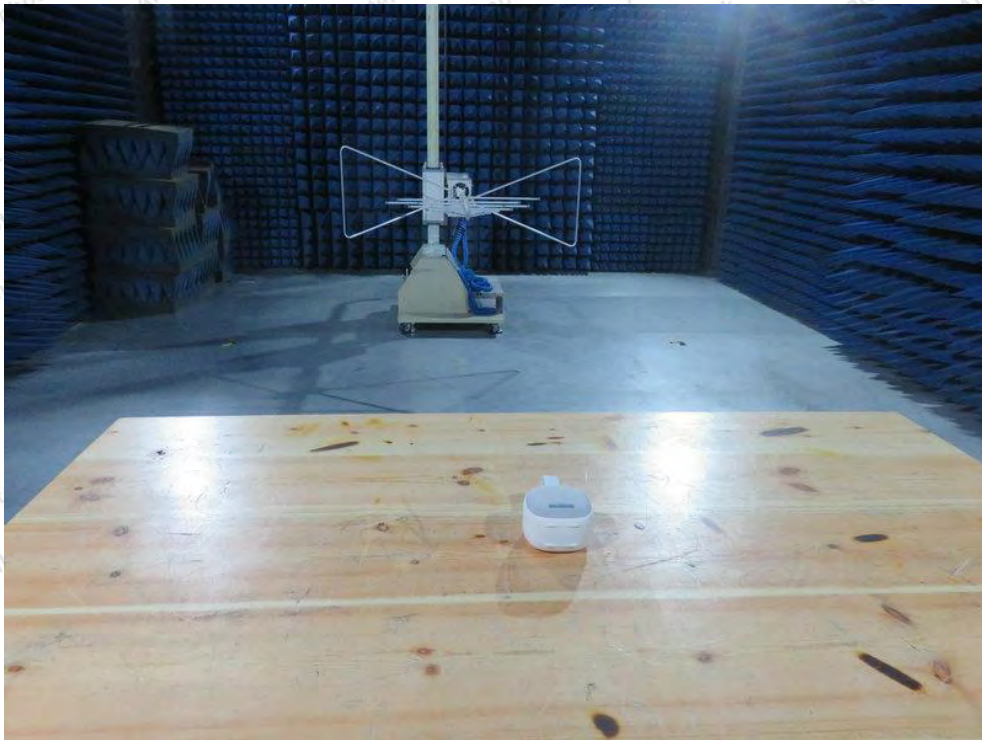
Photo of Radiation Emission Test
