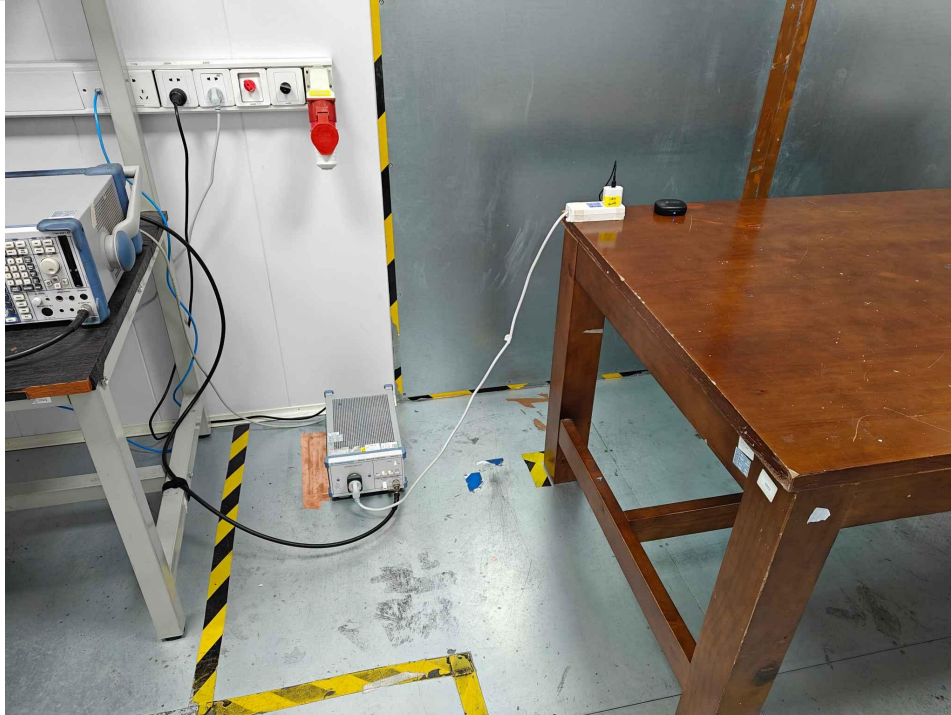
Conducted emissions at AC power line (150kHz-30MHz)
