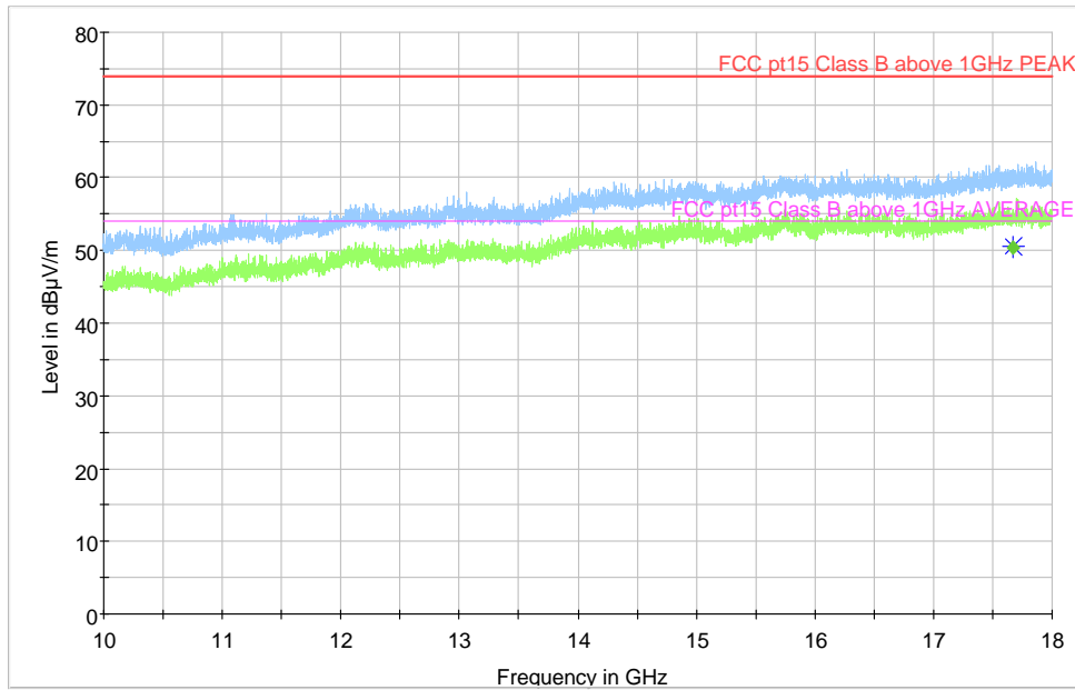
10 to 18GHz, Middle Channel, 2440MHz, X Orientation
