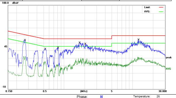
Site Phase: N Temperature: 26 Limit: FCC Part 15B\_(0.15-30MHz) \_Main\_QP Power: AC 120V/60Hz Humidity: 56 %
