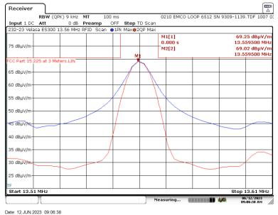
6.1.2. Worst Case Field Strength of the Fundamental – Perpendicular Antenna
