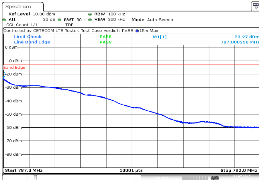
Plot 2: Highest channel, QPSK modulation
