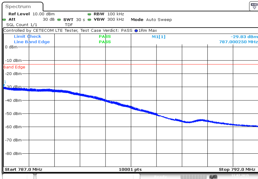
Plot 4: Highest channel, 16 – QAM modulation
