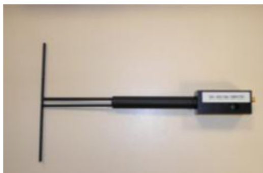
Figure 1 – Satimo COMOSAR Validation Dipole
