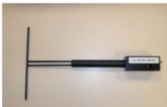
Figure 1 – Satimo COMOSAR Validation Dipole
