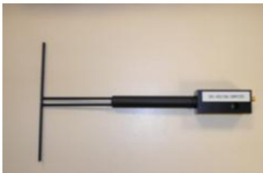
Figure 1 – Satimo COMOSAR Validation Dipole
