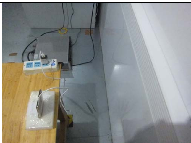
Conducted Emissions Test Setup Side View
