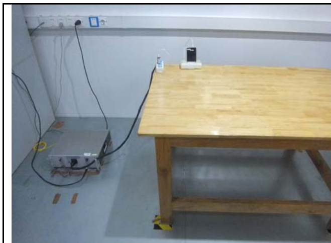
Conducted Emissions Test Setup Front View
