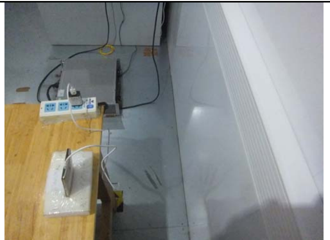
Conducted Emissions Test Setup Side View
