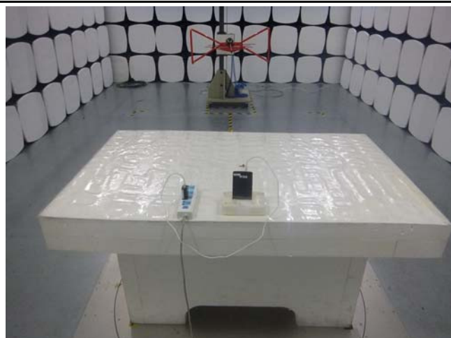
Conducted Emissions Test Setup Front View
