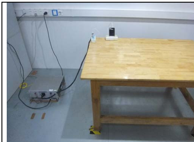
Conducted Emissions Test Setup Front View
