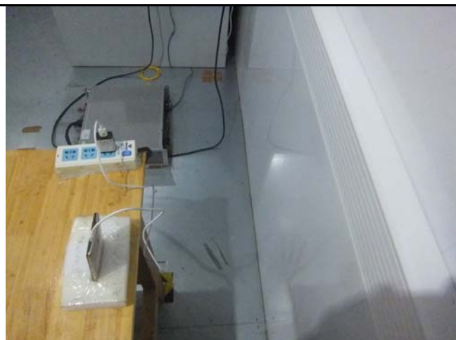
Conducted Emissions Test Setup Side View
