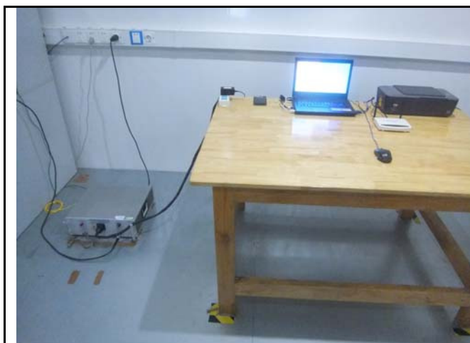
Conducted Emissions Test Setup – Front View
