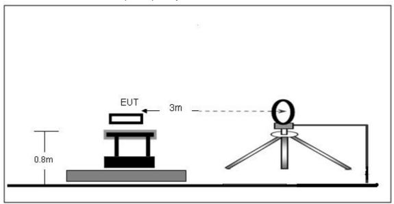
(B) Radiated Emission Test-Up Frequency 30MHz~1GHz
