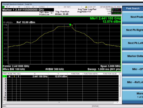
GFSK MIDDLE CHANNEL, CARRIER LEVEL
