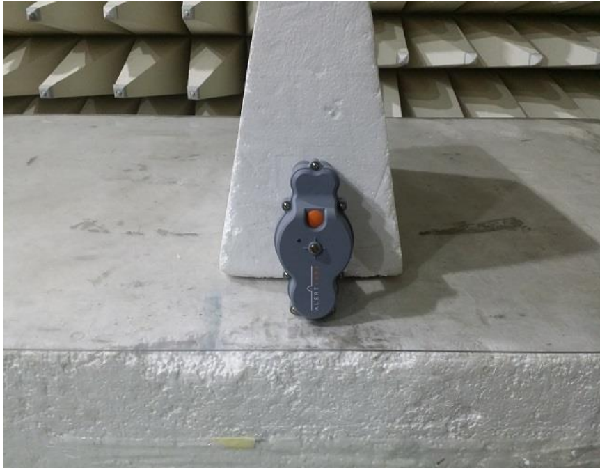
Photograph No.4 Setup for spurious emission field strength measurements, EUT close view
