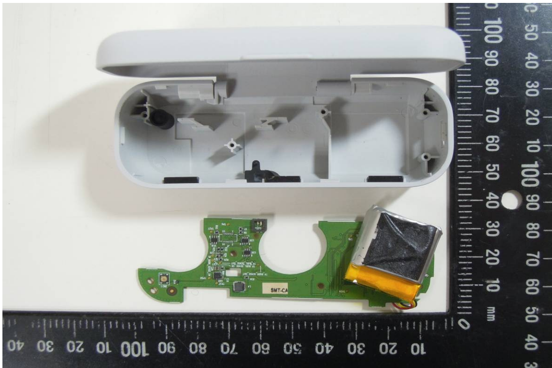
Open View of EUT – 4 (Charging Case)
