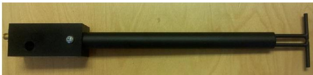
Figure 1 – MVG COMOSAR Validation Dipole
