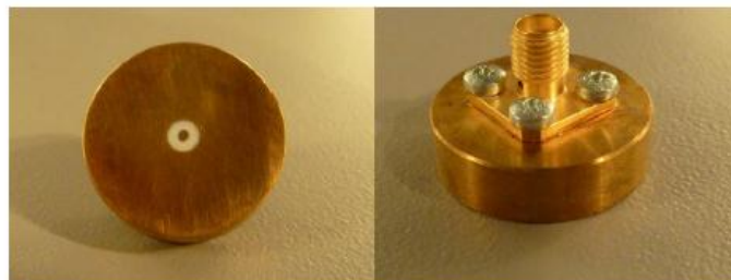
Figure 1 – MVG LIMESAR Dielectric Probe
