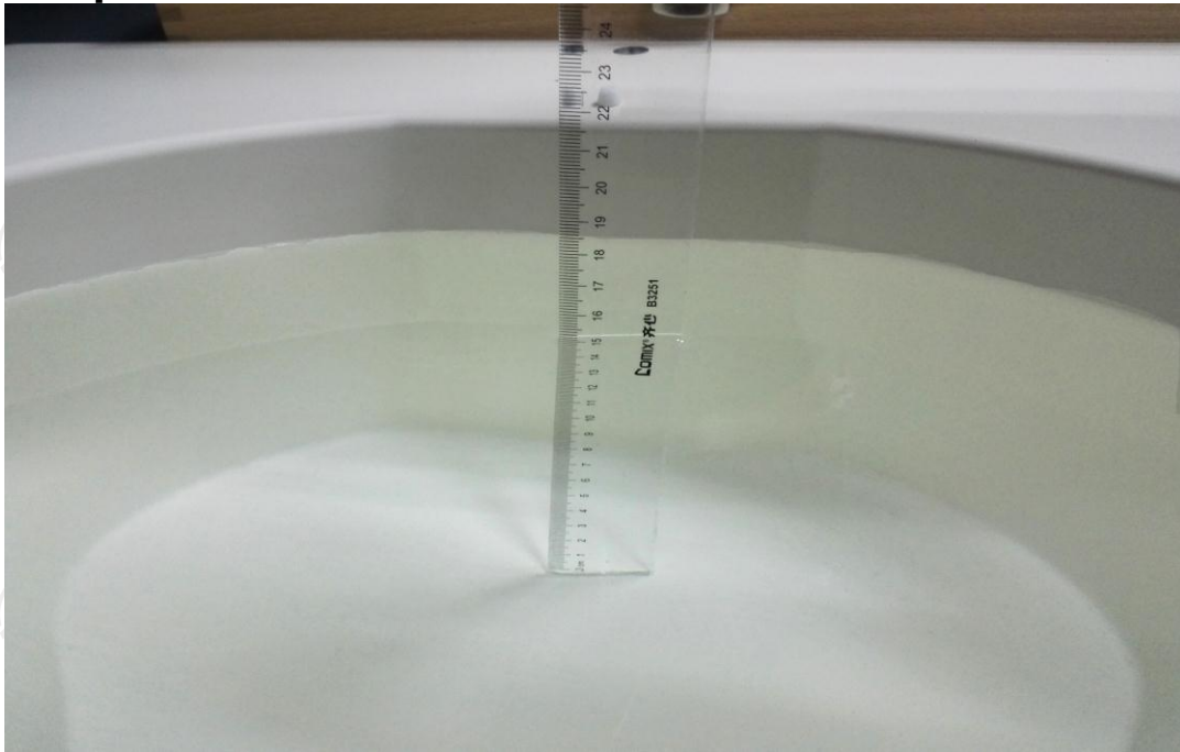
The Body Liquid of 2450MHz (15.3cm)
