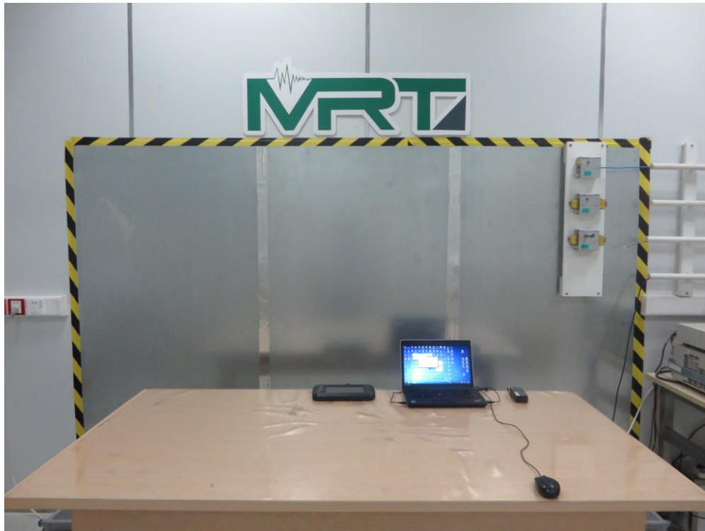
Description: Back View of the Conducted Emission Test Setup for 0.15kHz ~ 30MHz
