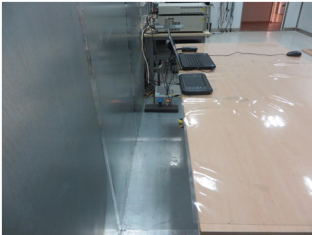
Description: Back View of the Conducted Emission Test Setup for 0.15kHz ~ 30MHz
