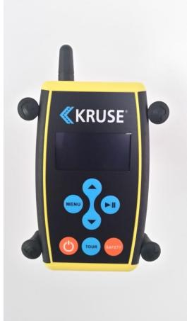
3. Turn on the KRUSEGO Tour Master using the ORANGE Power button at the bottom left of the keypad. The KRUSEGO Tour Master will now display "SYSTEM READY". Push the BLUE "TOUR" Button. The display will now read "SELECT TOUR" with the default "NONE". Push the ARROW UP button until the desired tour is reached. Press the PLAY/PAUSE Button and the display will now read "ON TOUR" for the selected tour. Shortly the screen will blink intermittently; this is "power save mode" to save battery power.
