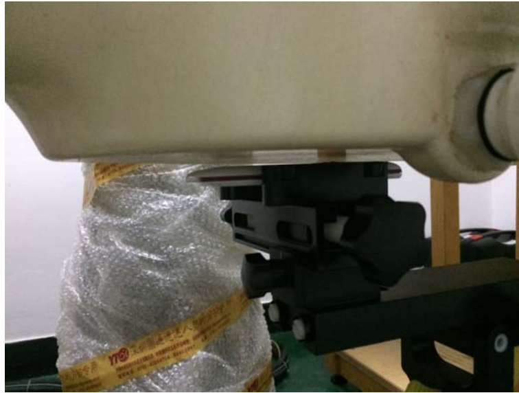
5mm Body-worn Rear Setup Photo
