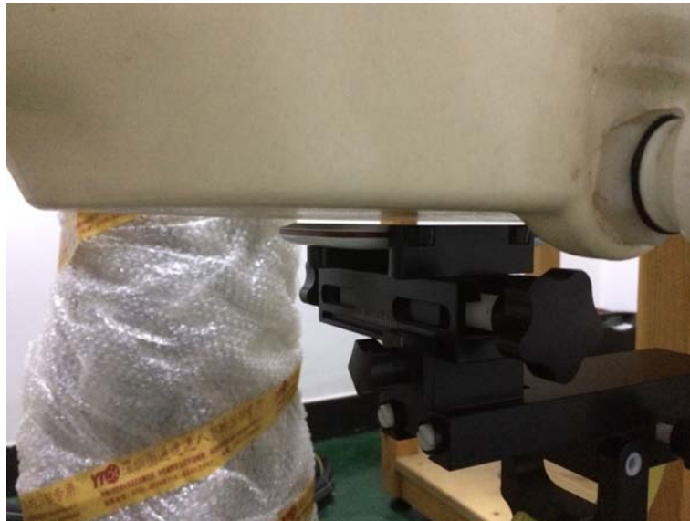
5mm Body-worn Front Side Setup Photo
