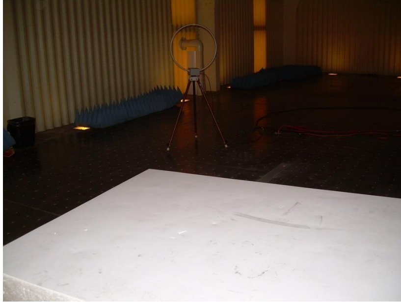
Photograph 3: View of Loop Antenna Placement for measurement of frequencies below 30 MHz
