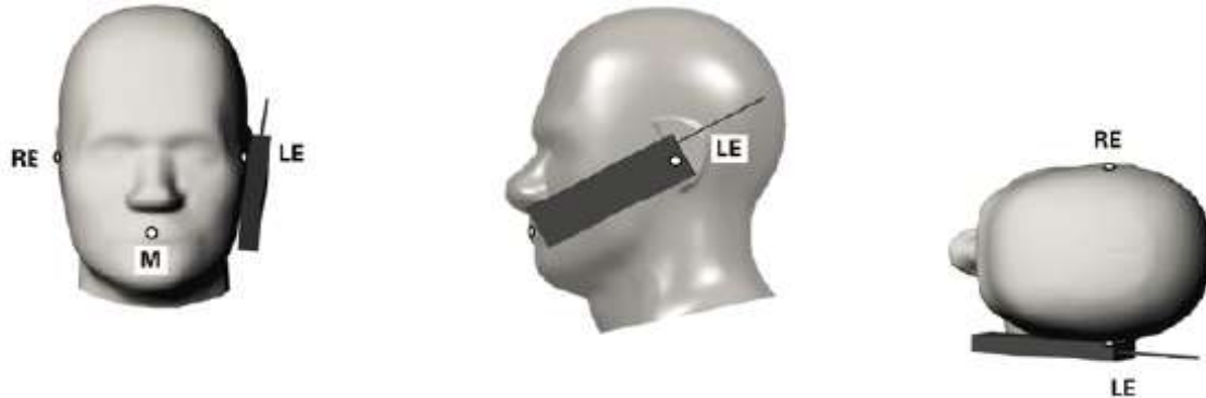
Fig. 11.3 Illustration for Cheek Position
