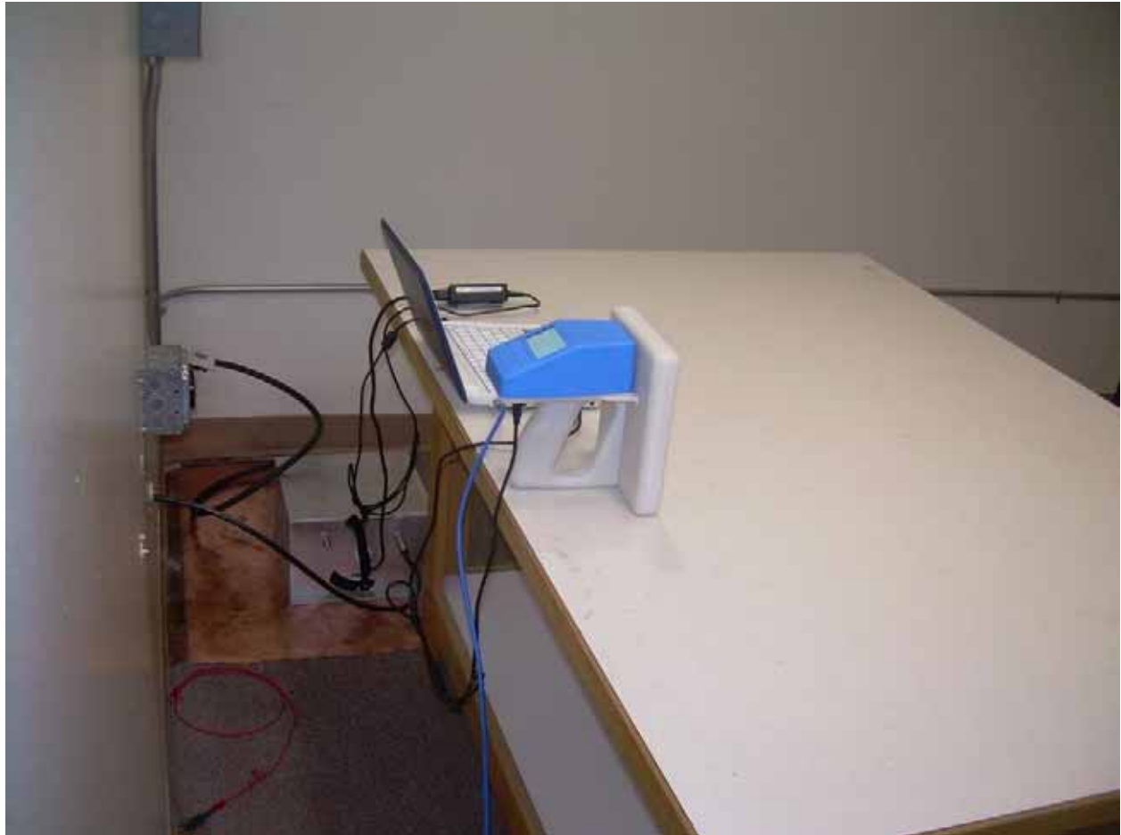
Photograph 9 – Back View Conducted Disturbance Worst Case Configuration
