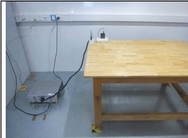
Conducted Emissions Test Setup Front View
