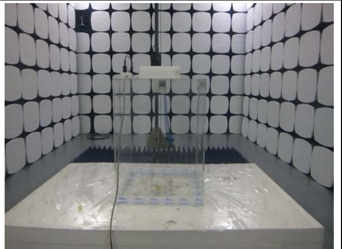
Radiated Spurious Emissions Test Setup Above 1GHz
