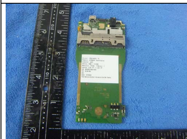
Mainboard with Shielding - Front View
