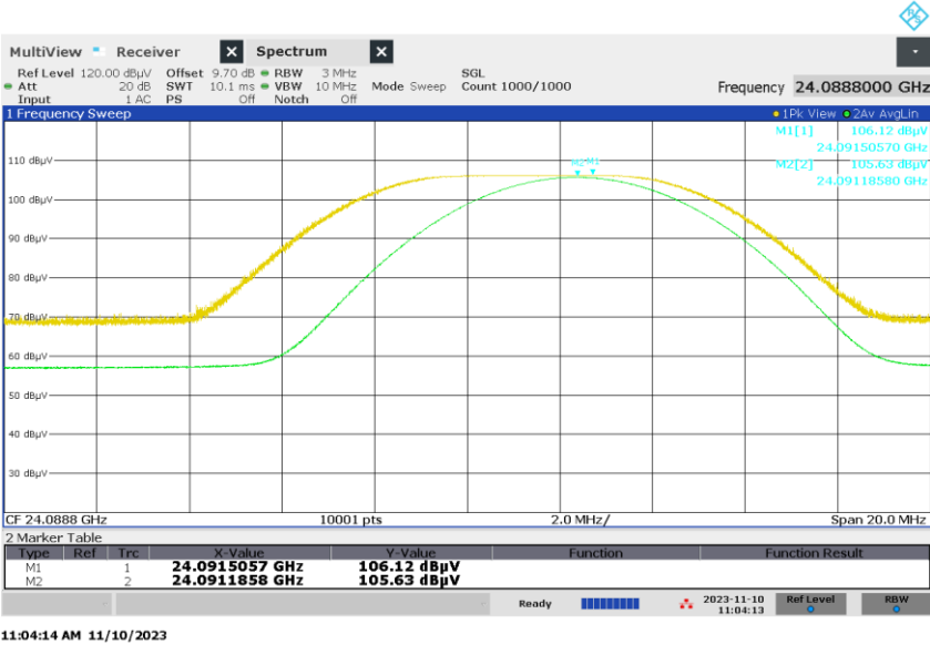
Figure 14: Field Strength of Fundamental, Spectral Diagram, Mode A
