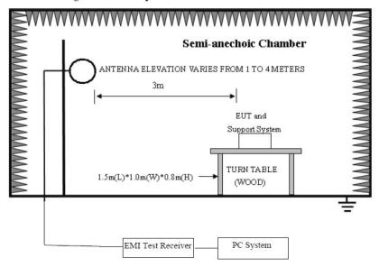
In 3m Anechoic Chamber Test Setup Diagram for frequency 30MHz-1GHz
