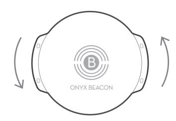
Twist the top of the case in the indicated direction open (counterclockwise). To separate the top from the bottom part of the enclosure.
