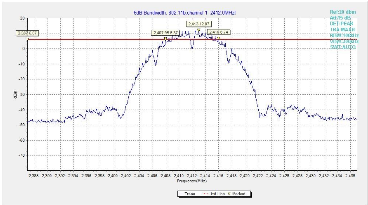
Fig.A.4.1 Occupied 6dB Bandwidth(802.11b,Ch 1)
