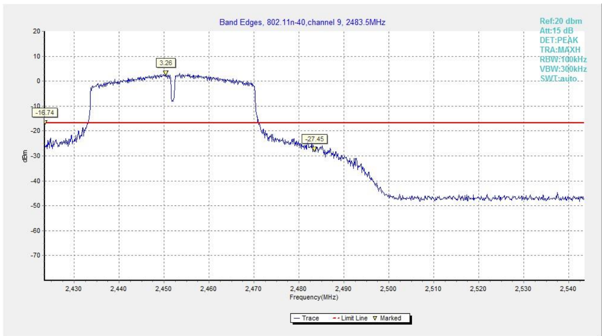
Fig.A.5.8 Band Edges (802.11n-HT40, Ch 9)
