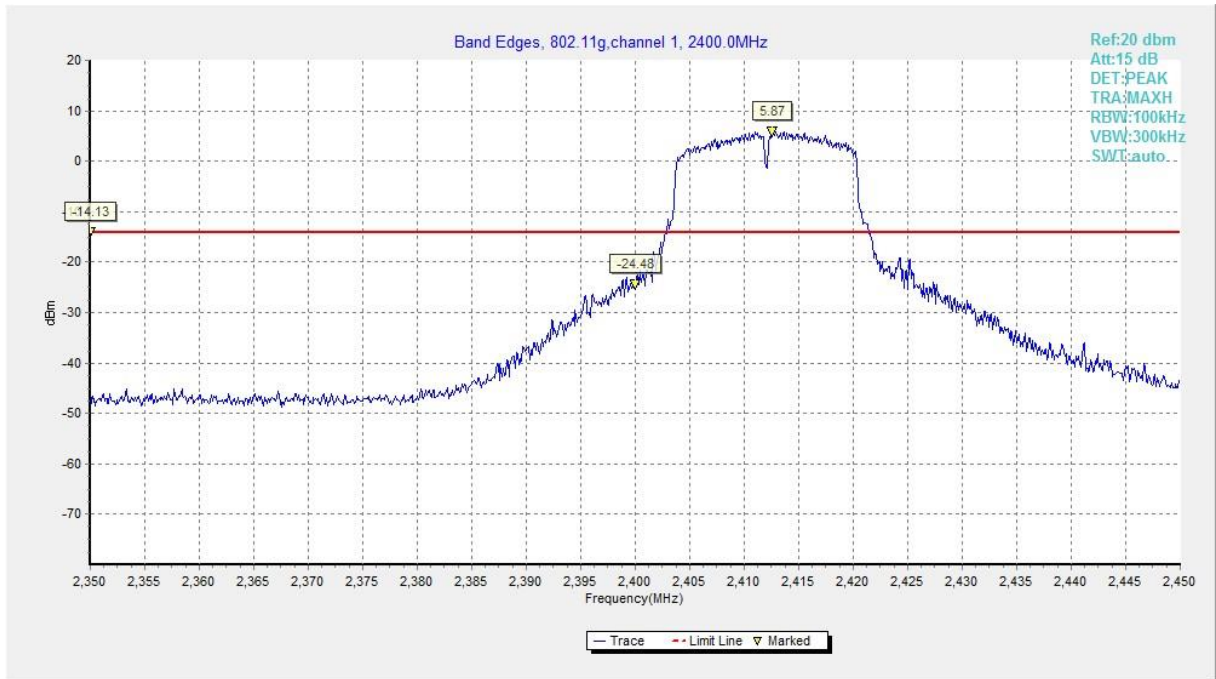
Fig.A.5.3 Band Edges (802.11g, Ch 1)
