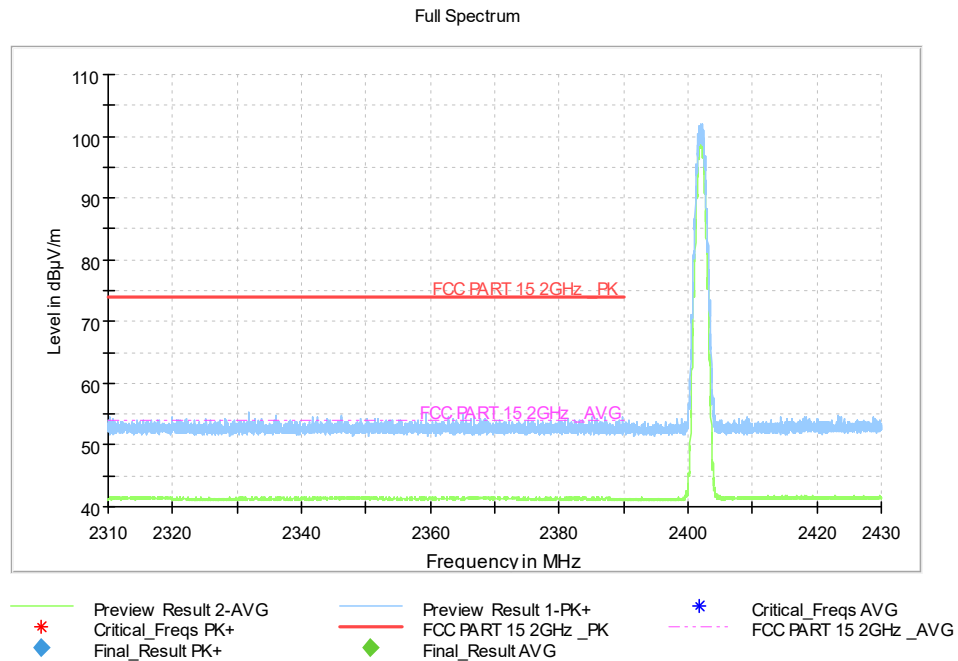
Fig.13. Frequency Band Edges: GFSK, Channel 0, Hopping Off, 2.31 GHz – 2.43GHz
