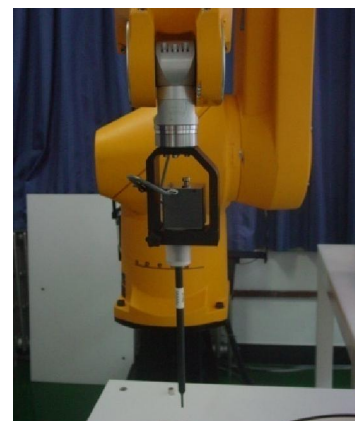
Picture C.2 Near-field Probe
