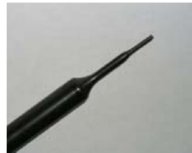
Picture C.2 Near-field Probe
