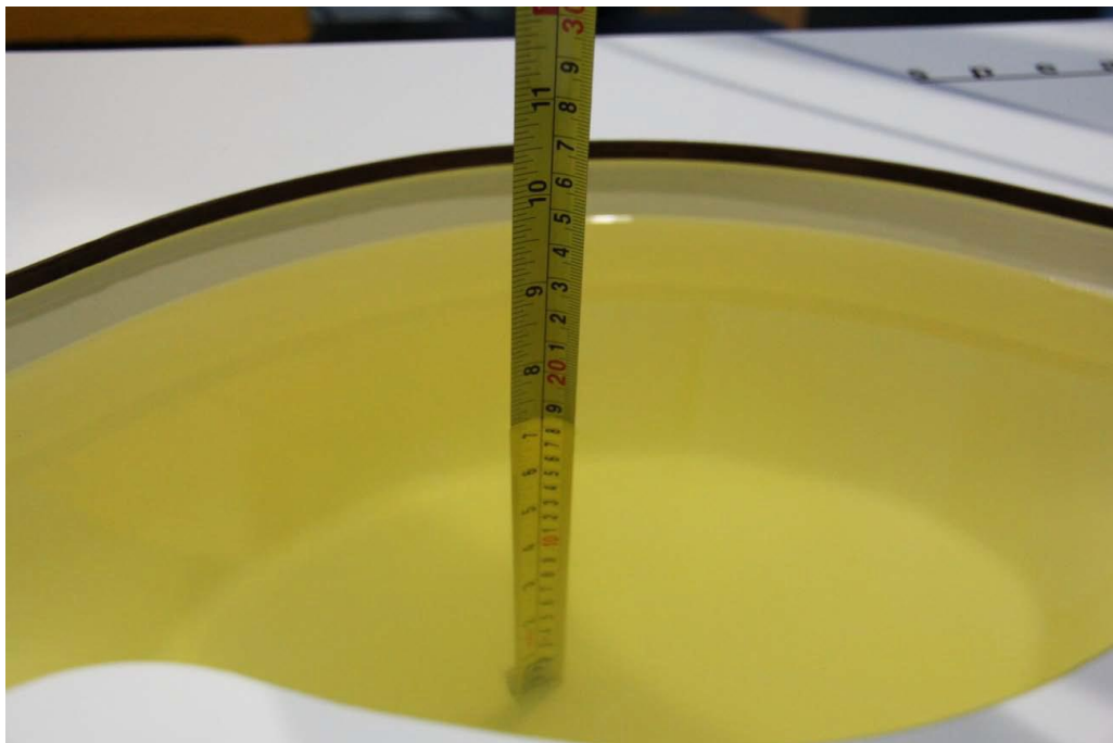
Picture 7-4: Liquid depth in the Head Phantom(2450MHz)
