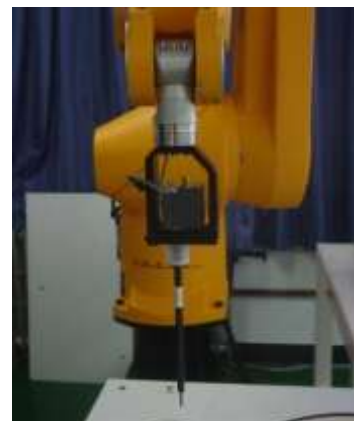
Picture C.3 E-field Probe
