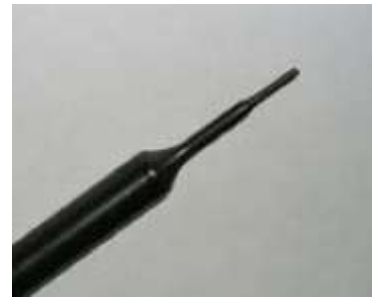
Picture C.2 Near-field Probe
