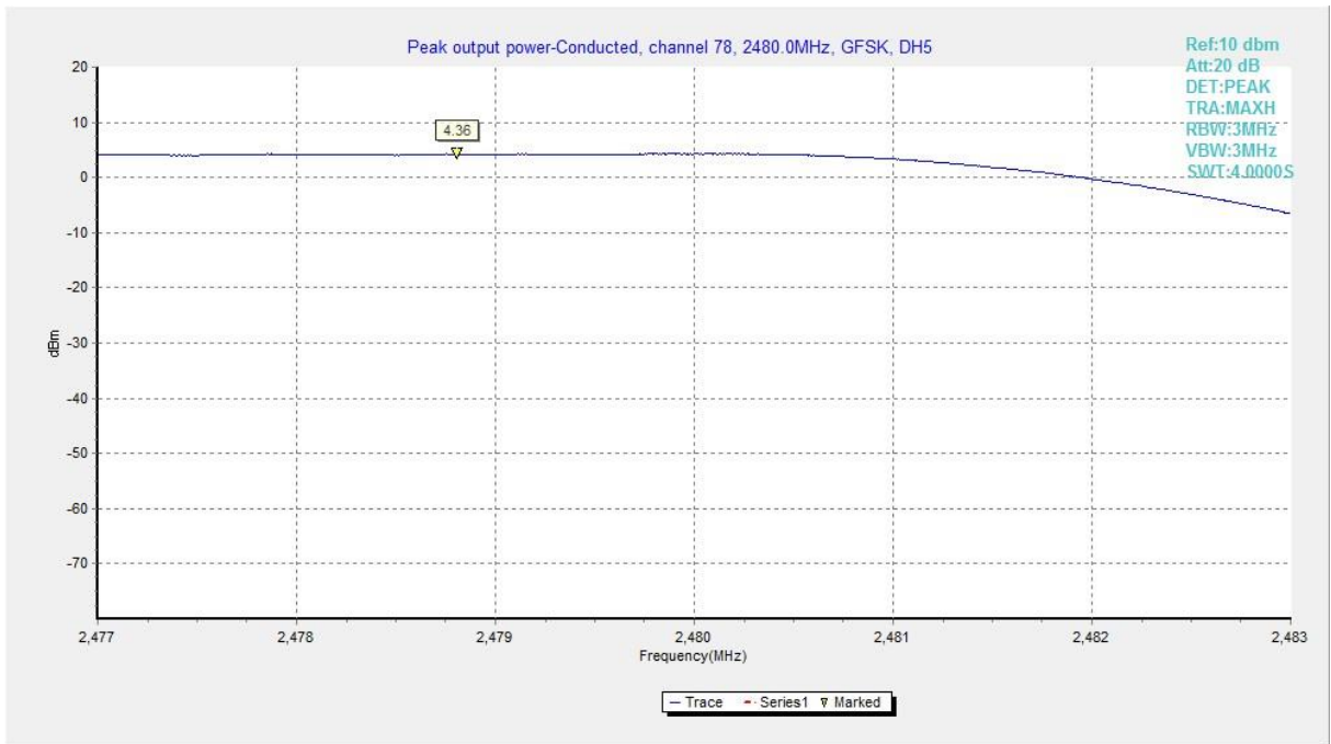
Fig. 3 Maximum Peak Output Power (GFSK, Ch 78)
