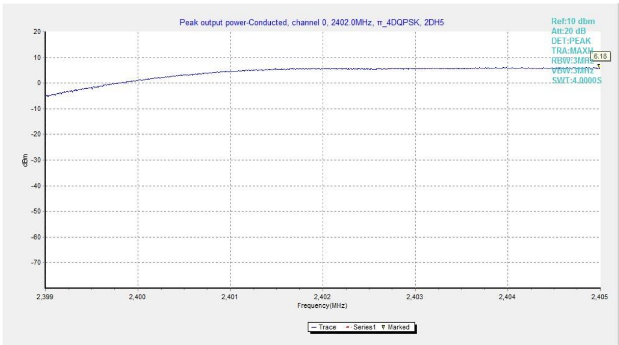
Fig. 4 Maximum Peak Output Power ( \pi/4 DQPSK, Ch 0)
