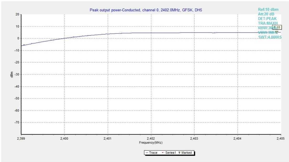
Fig. 1 Maximum Peak Output Power (GFSK, Ch 0)
