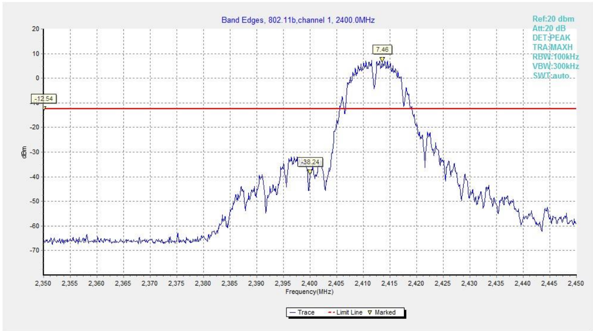
Fig.19 Band Edges (802.11b, CH 1)
