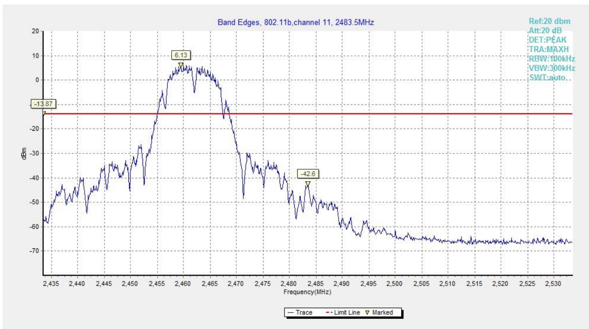
Fig.20 Band Edges (802.11b, CH 11)
