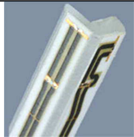
Fig 5.2 Photo of E-field Probe
