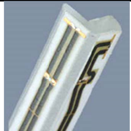
Fig 5.2 Photo of E-field Probe
