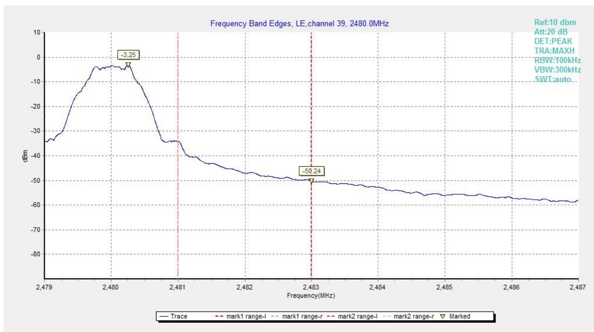
Fig.8 Band Edges (Ch 39)
