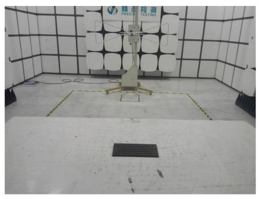
RADIATED EMISSION TEST SETUP ABOVE 1GHz
